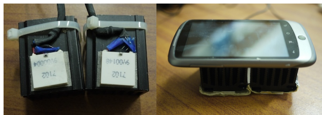
Fig. 1. Peltier modules used to produce thermal icons (left); attached to back of mobile (right).
